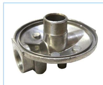
Filter Holder Item. No. TSFS-GL-2 Material: aluminum In/outlet: 1" Size: 1 1/2"-16UNF
